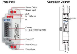
. By flashing, the LED on the front panel makes it possible toobserve whether the measuring is active or not.
