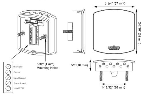
Note: Internal Thermistor, one side common to signal ground
